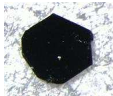
Fig. 2: Micrograph of a chiral magnetic crystal of \text{CrNb}_3\text{S}_6 .
